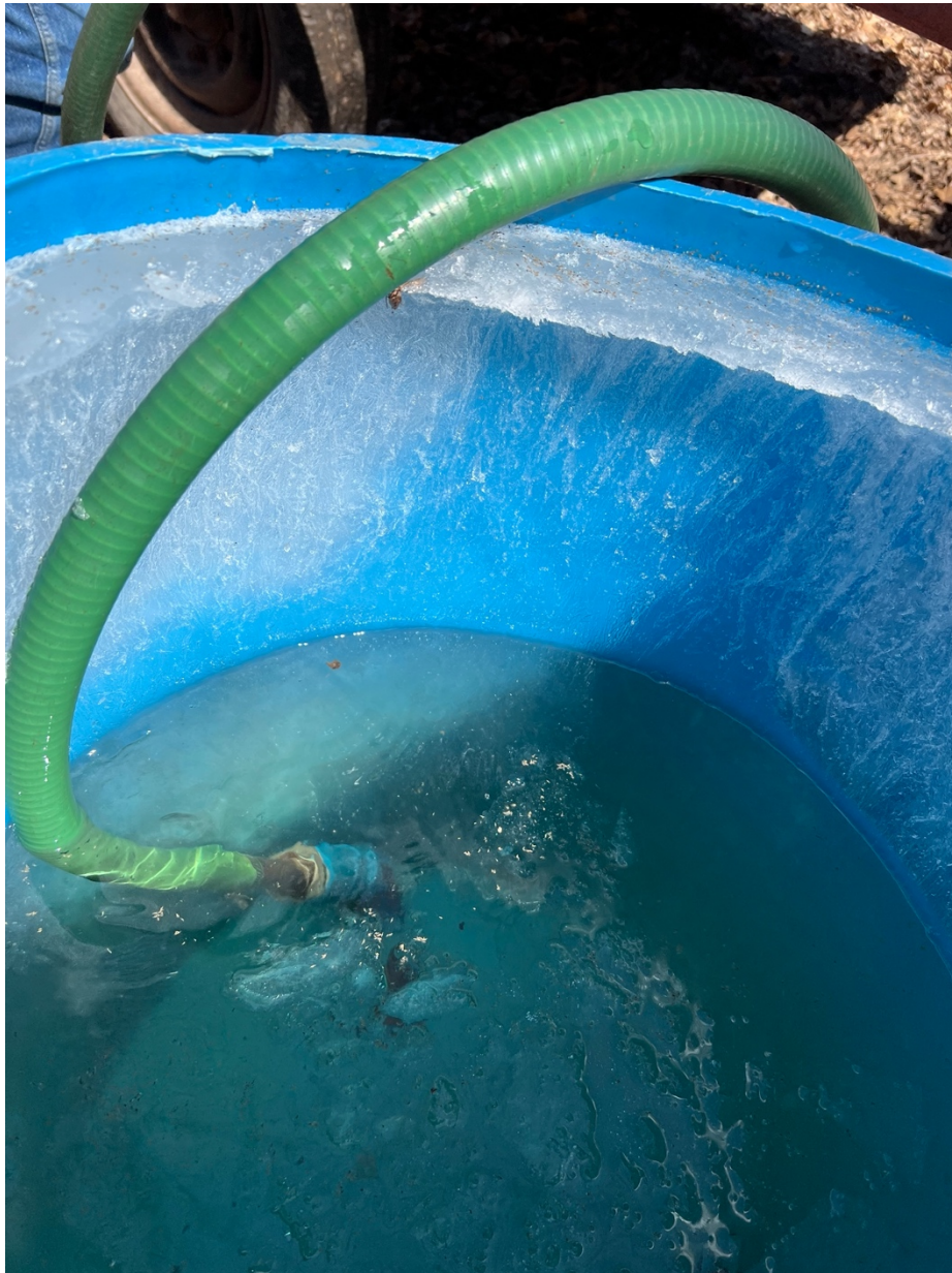
Figure 20. Thick layer of ice that formed in a storage barrel before it could be emptied. Photo taken on March 26, 2022.
