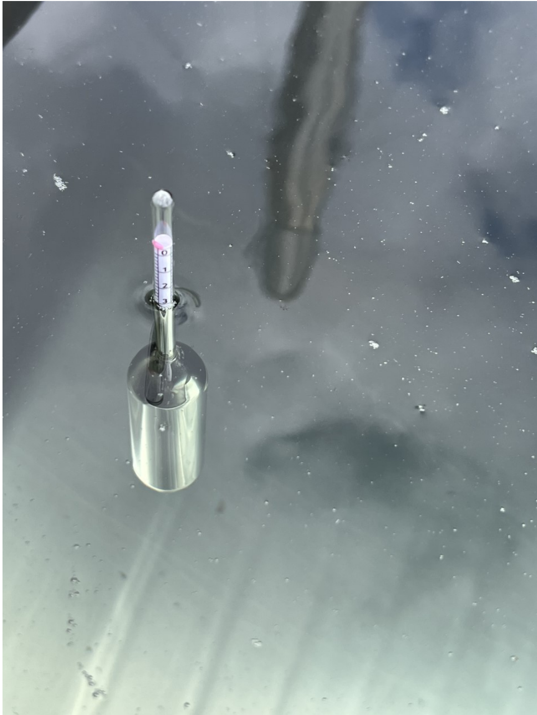
Figure 27. Hydrometer floating in sap in one of the storage tanks showing the beautiful clarity and high sugar concentration.
