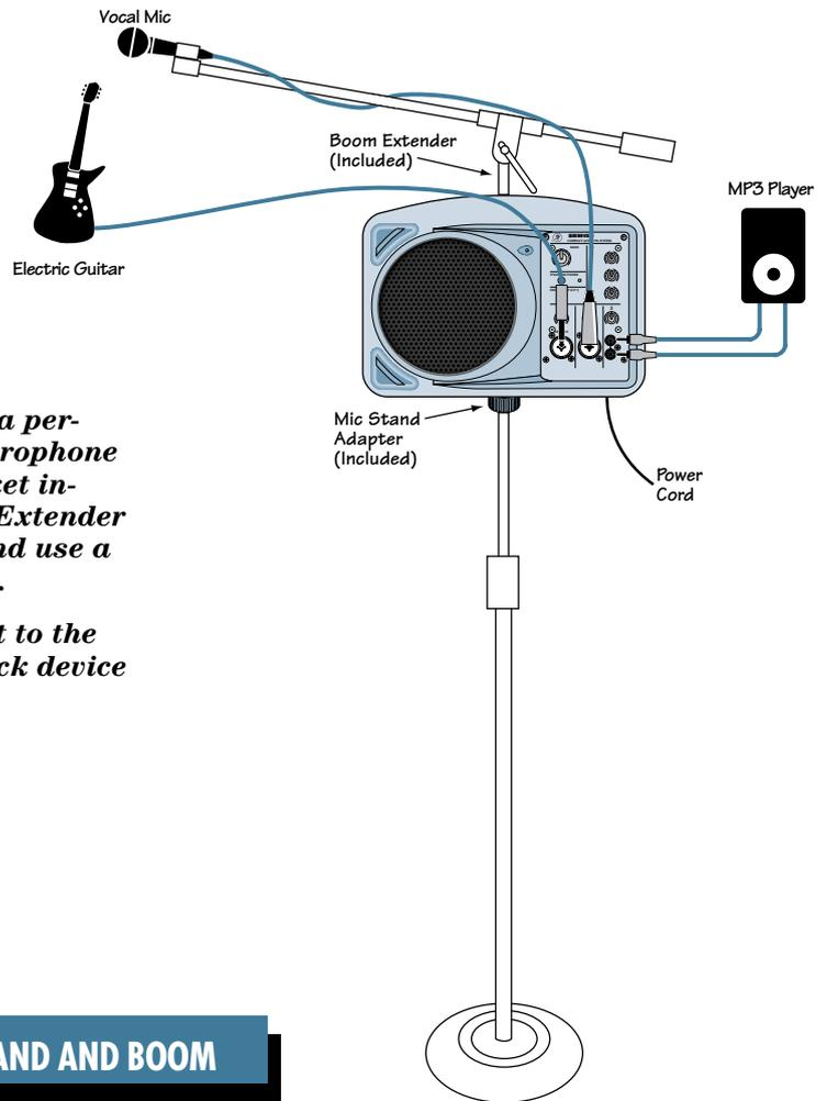
*This illustrates how to use the SRM150 as a personal monitor. Mount the SRM150 on a microphone stand using the Mic Stand Mounting Bracket included with the SRM150. Attach the Boom Extender (also included) to the top of the SRM150 and use a microphone boom to hold your microphone.*
