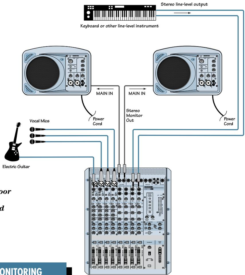
*Two SRM150s are used as floor monitors to provide a stereo monitor mix for the keyboard player.*
