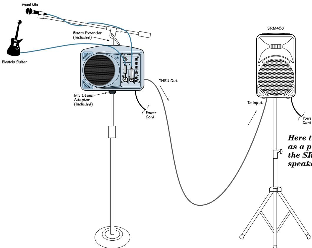
*Here the SRM150 is used as a personal monitor and the SRM450 is the main PA speaker.*
